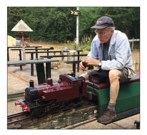
NLSME Club loco "*Butch*" on first run after significant repair undertaken by Mike F. Loco features a new copper (welded) boiler, grate and ash pan.
